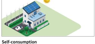
Extra PV power charges the battery. When there is little to no PV power, power should be taken from the battery first to minimize power taken from the grid.
